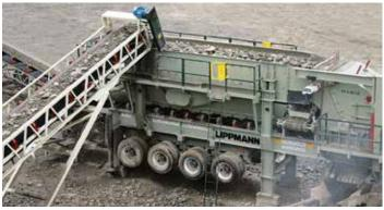
Tough aggregate is no match for the four blow bars. Day in and day out consistent gradation and greater top sized control are reliably delivered.
