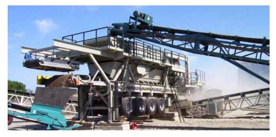
The 5165is-w is a secondary impact crushing plant perfectly suited to be paired up with a primary jaw crusher. The screen plant and impactor are perfectly paired to size the material for your required specification. The impactor is heavy-duty enough to handle recycle material and will withstand the tramp metal that might be present from the primary crusher. The top cross conveyor is extended to ensure you can take both products out on the same side of the plant.
