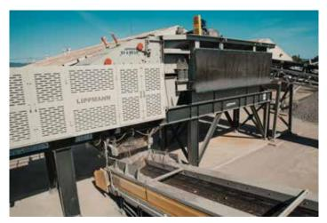
As a secondary crusher, this heavy duty impactor handles recycled material and will withstand any tramp metal that makes it through the primary crusher.
