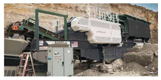
This plant is specifically designed to process primary feed in the toughest of applications with an extremely high production rate and minimal downtime. With a high reduction ratio, this plant is ideal for aggregate and recycle applications and accepts a front discharge conveyor and a return chute to be paired up with a screen plant to make a closed circuit plant as applications require it.
