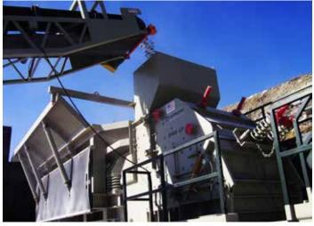
With two adjustable breaker plates for setting adjustment, this impactor is ideal for both primary aggregate and recycle applications.
