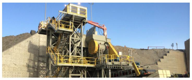
This primary crushing station is designed for heavy-duty and high production applications. With it handling 100-ton trucks this plant is capable of 1800-2200tph. Lippmann designs customer primary stations that will fit their needs and demands. Keeping safety in mind, Lippmann has designed these plants with plenty of clearance to easily maintain this large equipment and provide optimum uptime for the customer by allowing material to flow freely.
