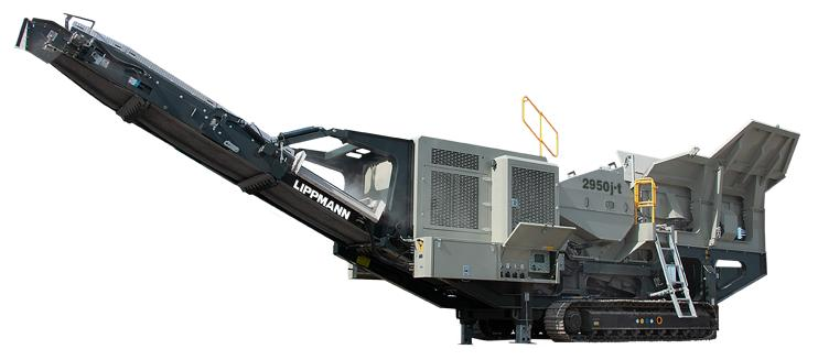
Maximum productivity is delivered through the 50" x 29" single toggle jaw with speeds that lead to better reduction and material being processed faster through the crushing chamber. This plant has enhancements to the jaw box including heavier flywheels and optimization for all crushing applications. With a class-leading throughput, capacity and largest stockpile height in its category, the 2950j-t brings even more power and productivity together in one machine.
