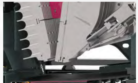
The large gap between crusher discharge and main conveyor belt, paired with wide main and side conveyors result in an optimized material flow.
