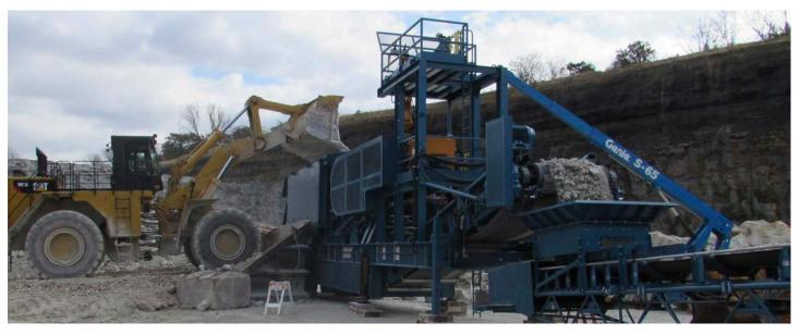
The 3862j-w is one of the newer jaw crushers in the Lippmann fleet designed to give you a little more gape but maintain the aggressive nip angle resulting in a higher rate of production. The plant features a wide 62" feeder with a 10' grizzly section ideal for cleaning material prior to going into the crusher. This will increase efficiency and production going through the jaw crusher.
