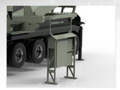
Hydraulically-removable electric cabinet reduces vibration to components.
