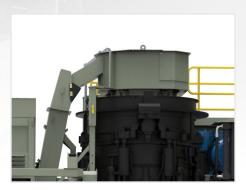
Overflow chute prevents spillage, keeping product moving and maintaining a clean site.
