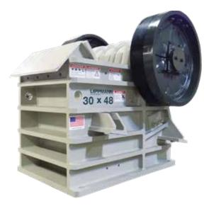
Our world-renowned jaws lie at the core of Lippmann's product offering and have been manufactured in Milwaukee, WI, since 1923. Fabricated with extra heavy ribbed steel plate construction, Lippmann jaw crushers have proven time and again they provide maximum strength, durability, and reliability at the lowest cost of ownership in the industry.
