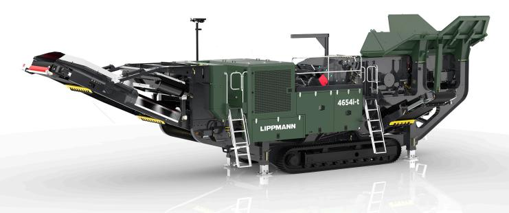
Heavy duty track mounted crusher with following features: 1200mm (48") diameter x 1350mm (53") wide impactor, 510 Hp (380 kW) Volvo D13 Stage V engine / 516 Hp C13 CAT LRC / 536 Hp C13 CAT, tracked, integrated hydraulic folding hopper, integrated hydraulic folding stockpiling conveyors, I-beam plate fabricated chassis construction, open chassis design for ease of maintenance, fast setup time, and vibrating feeder under crusher discharge.
