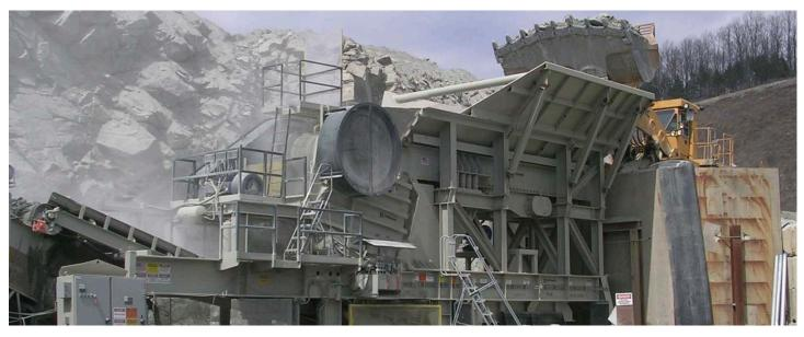
This jaw plant is designed for in-pit crushing, high capacity applications and provides unmatched production and reliability in the market. It features an options hammer and hopper extensions capable of handling large front end loaders or trucks and is specifically designed to handle 1000+ tons per hour making sure there is enough capacity in the hopper and conveyor to be able to obtain this.
