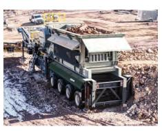
Rugged Lippmann feeder is capable of handling side or rear loading from various types of equipment.
